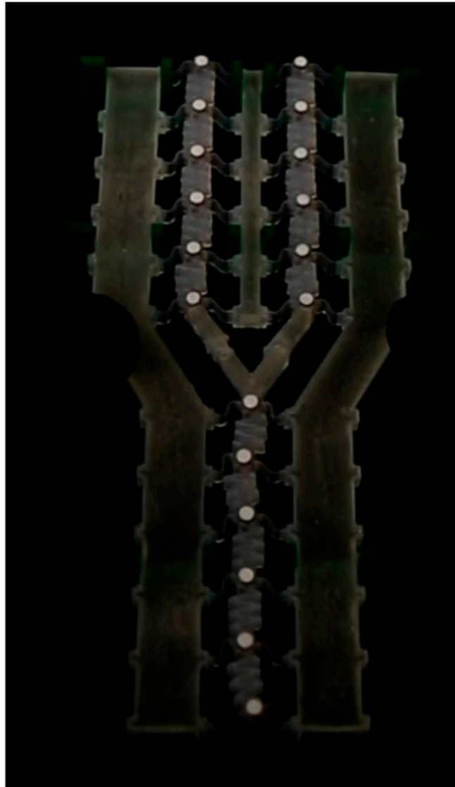
Movie S6. A bifurcated system in which functional “and” behavior is realized through the control of the spacing in the output chain ( d_{\text{out}} = 16.7 mm). Both input chains must be activated in order for a pulse to propagate in the output chain.
