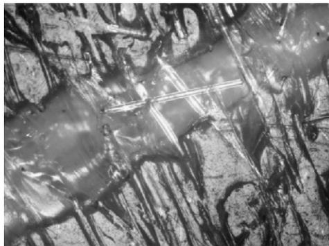
Fig. 1. A bridged fracture in short-glass-fiber-reinforced polypropylene.
