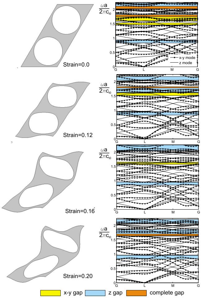
FIG. 5. (Color online) Phononic band gap structure for the oblique array of circular holes with  $r=4.335$  mm,  $a_x=10.97$  mm, and  $a_y=9.47$  mm ( $f_0=0.57$ ) at different levels of macroscopic nominal strain in the elastomer matrix ( $c_{l0}=32.2$  m/s). In-plane (labeled  $x$ - $y$ ) and out-of-plane (labeled  $z$ ) modes are reported together with the  $x$ - $y$ ,  $z$ , and complete band gaps. The points  $G$ ,  $L$ , and  $M$  are defined in Fig. 2.
