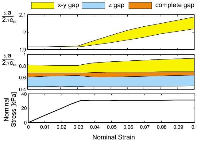
FIG. 4. (Color online) Phononic band gap (top and center) and nominal stress (bottom) vs nominal strain for the square array of circular holes.
