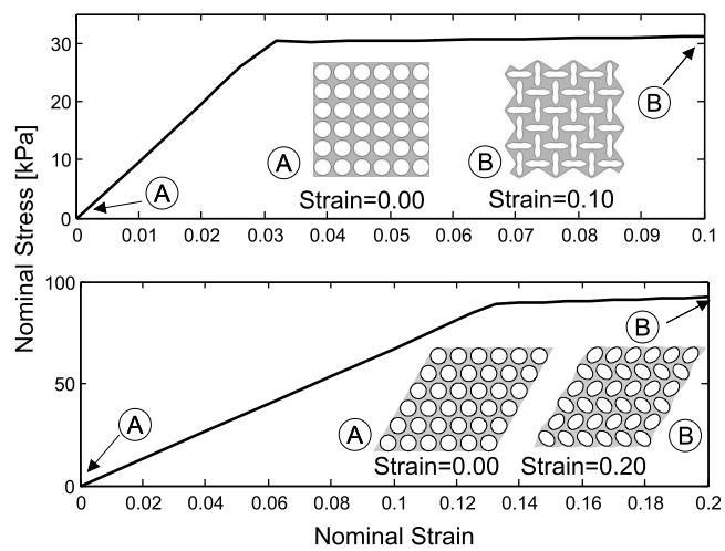
FIG. 1. Nominal stress vs nominal strain curves during axial compression in the vertical direction for the square (top) and hexagonal (bottom) arrays of circular holes. The departure from linearity is the result of an elastic buckling in the microstructure that triggers a pattern transformation.
