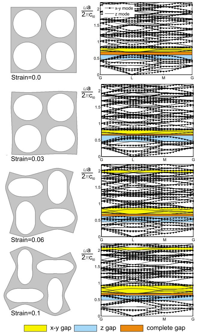
FIG. 3. (Color online) Phononic band gap structure for the square array of circular holes with  $r=4.335$  mm and  $a_x=a_y=9.97$  mm ( $f_0=0.59$ ) at different levels of macroscopic nominal strain in the elastomer matrix ( $c_{l0}=32.2$  m/s). In-plane (labeled  $x$ - $y$ ) and out-of-plane (labeled  $z$ ) modes are reported together with the  $x$ - $y$ ,  $z$ , and complete band gaps. The points  $G$ ,  $L$ , and  $M$  are defined in Fig. 2.
