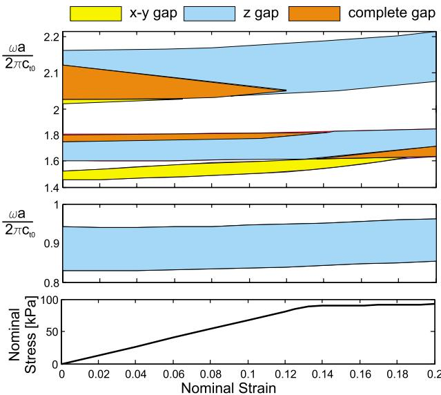
FIG. 6. (Color online) Phononic band gap (top and center) and nominal stress (bottom) vs nominal strain for the oblique array of circular holes.
