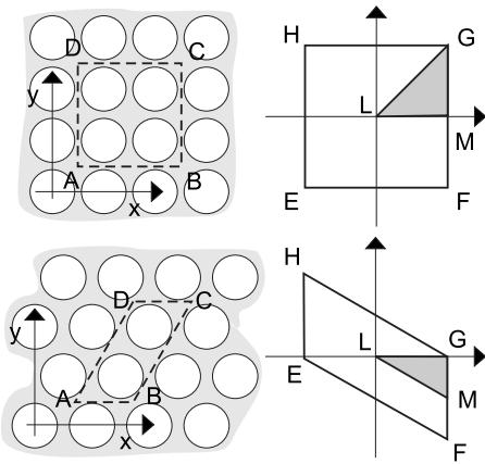
FIG. 2. Square (top) and oblique (bottom) infinite array of circular voids: cell in the direct lattice (left) and its corresponding in the reciprocal lattice (right). The perimeter of the gray area illustrates the contour along which the eigenfrequencies are plotted.
